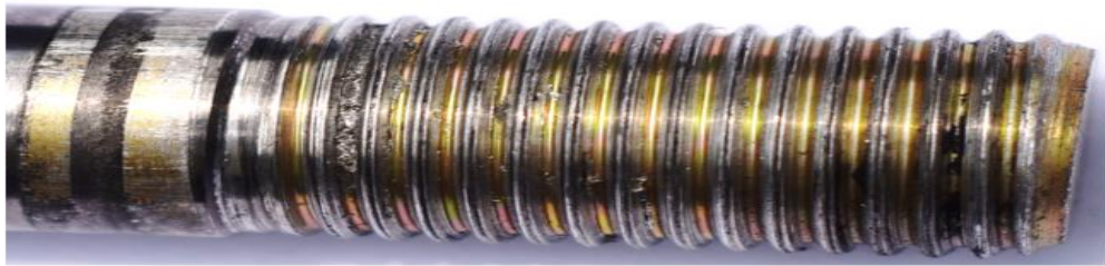
Thread damage on the bolt fastening at inboard landing gear bulkhead
