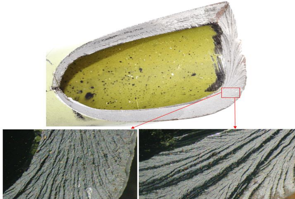
Slant, fibrous feature and chevron marks seen on the fracture surface
