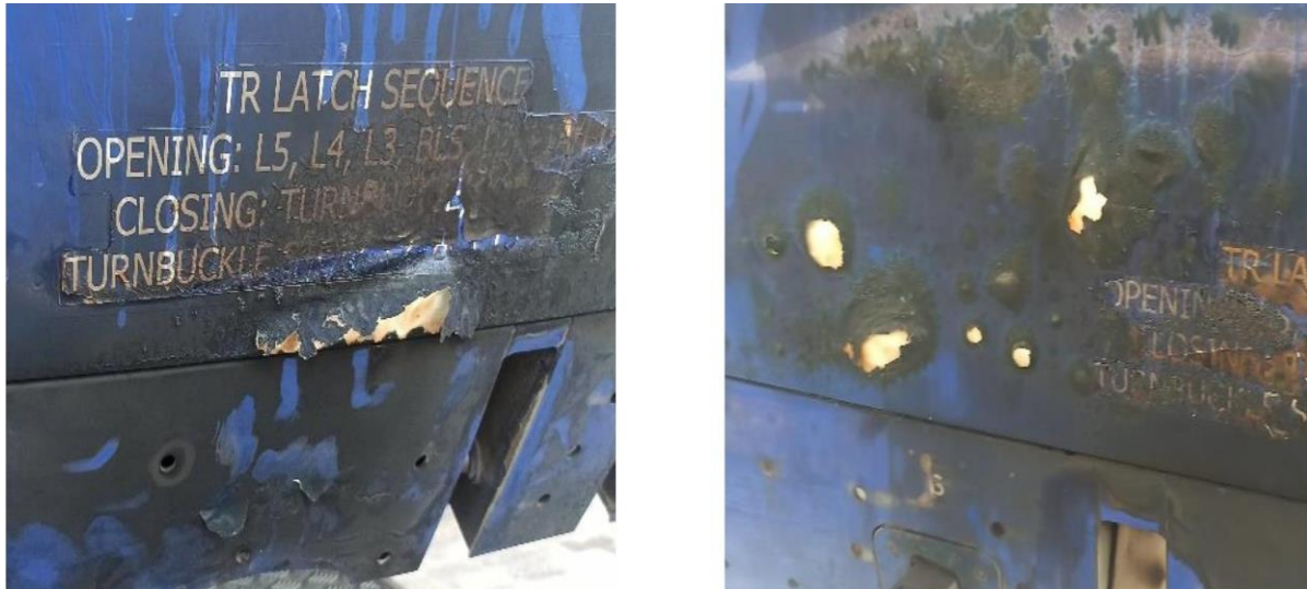
(Fig. 1.1: Paint peel on the Lower Section of Engine No.2 Thrust Reverser Cowling)
