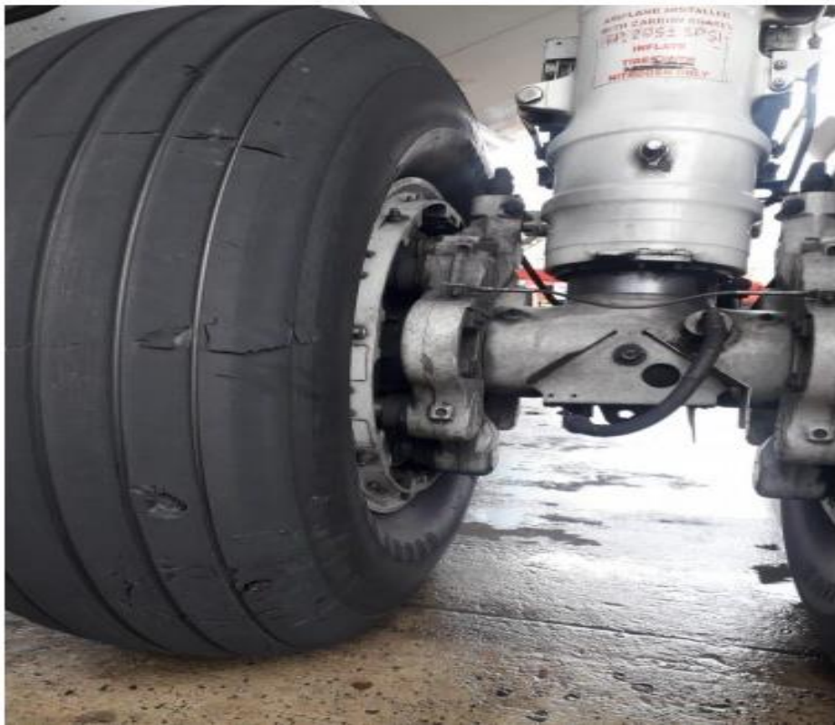
Cut Marks on no.3 main wheel tyre
