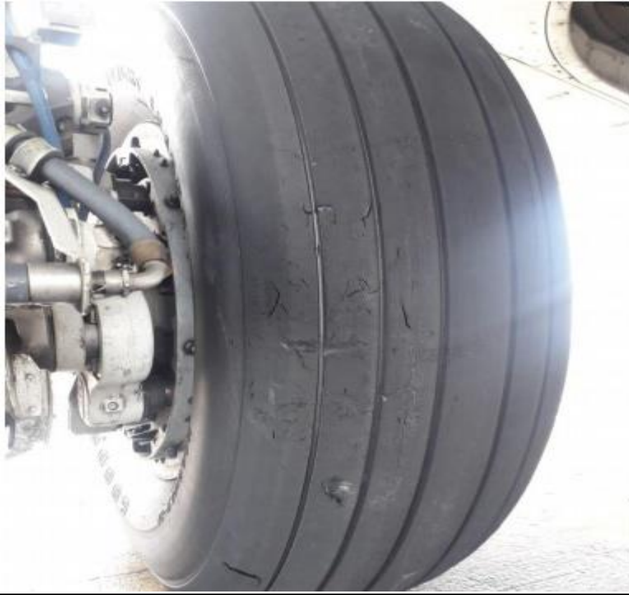
Cut Marks on no. 4 main wheel tyre.
