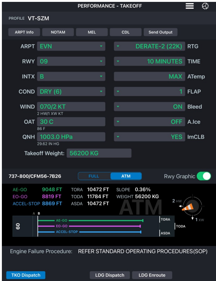
OPT input data and its output used for take-off from Yerevan (UDYZ)
