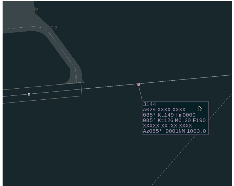
Radar playback image indicating position of SG9029 (11:50:12 UTC) at liftoff beyond TORA of RWY09.
