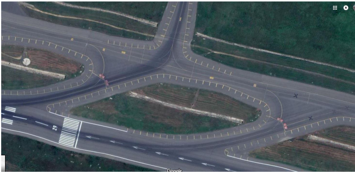
Fig.8:- Taxiways Z-z4 and Z3 with markings
