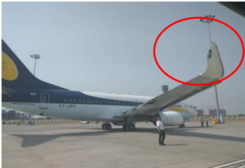
Fig.2:- Damaged winglet of VT-JGY
