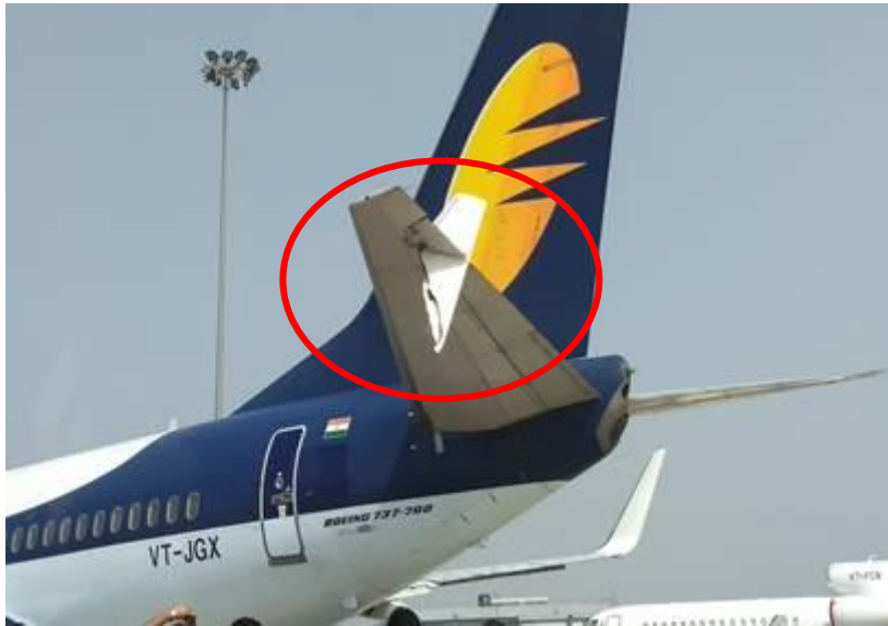
Fig.1:- Detached portion of winglet of VT-JGY intact with the elevator if VT-JGX
