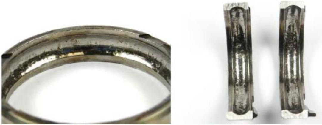
Figure 14: RDS Bearing outer ring Characterization (raceway & shoulders)
