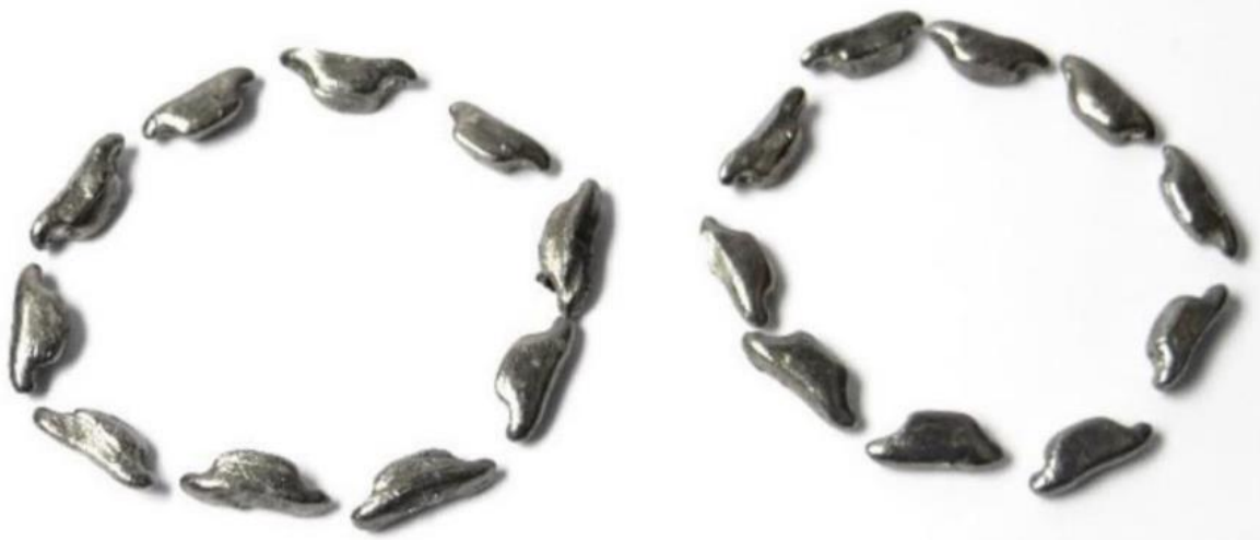
Figure 20: RDS Bearing Cage Characterization (cage fragmented)
