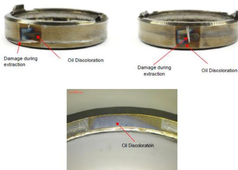
Figure 16: RDS Bearing Outer ring Characterization (Outer ring lateral face, TGB side)
