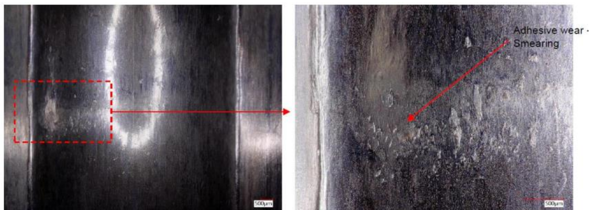
Figure 19: RDS Bearing Inner ring Characterization (raceway details)
