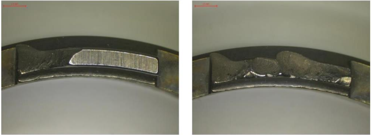
Figure 17: Fracture of anti-rotation pins (Outer ring lateral face, IGB side)
