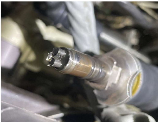
Figure 6: TM Magnetic Chip Detector
