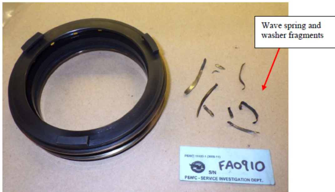
Figure 15: No.3 Carbon Seal wave spring & washer fragments
