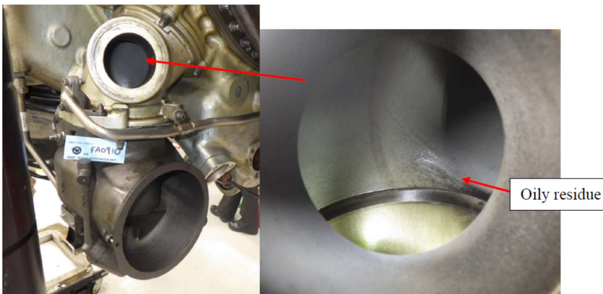
Figure 11: Oily P2.2 Interstage Bleed Valve
