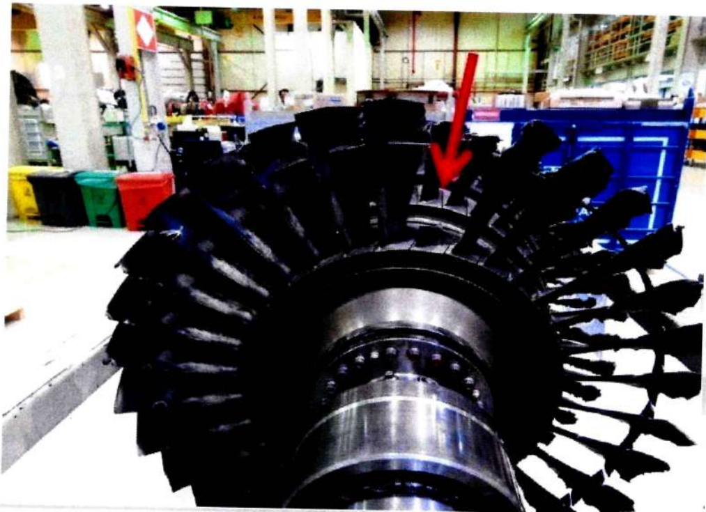
Fig. VII: HPC rotor blades with distortions/and quantity 01 blade broken off.
