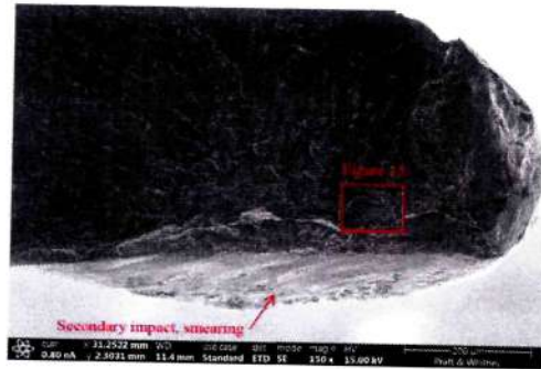
Fig. 12: SEM image of origin area, ~150x magnification. Large area of secondary impact damage smeared over approximate origin.
