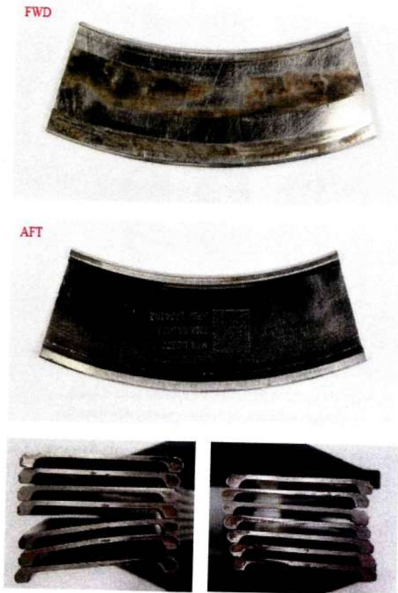
Fig. 19: Overall images of typical 3rd stage blade retaining plate forward side (top), aft side (middle), and retaining plate edge wear/deformation (bottom).
