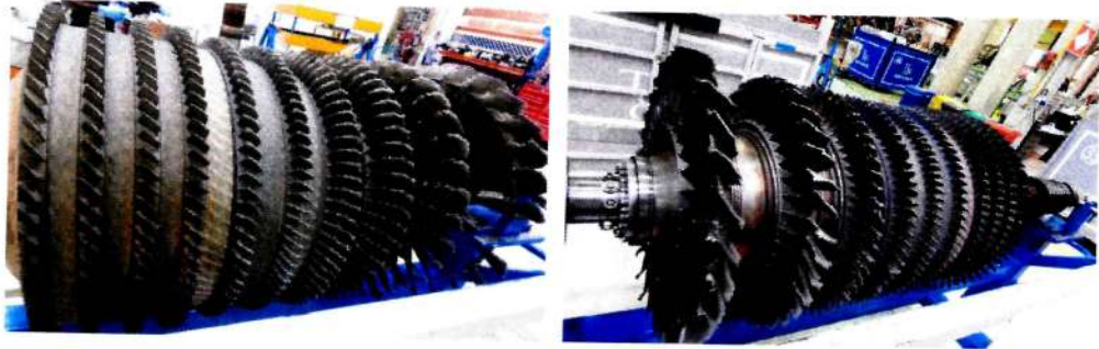
Fig. VI: HPC rotor blades with distortions
