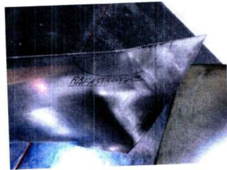
Fig. III: Damaged fan blade (bend on leading edge)
