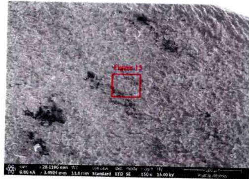
Fig. 14: SEM image of fracture progression, ~150x magnification
