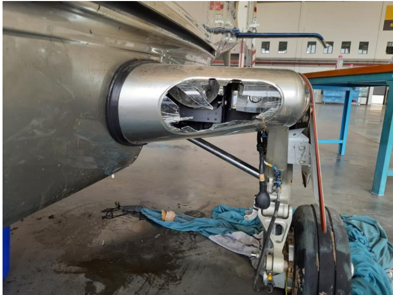
(Fig. 22: LH& RH Sponson Landing/taxi Light Glass found Broken)
