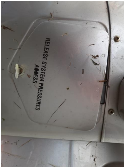
(Fig. 20: Utility accumulator access panel Deformed)
