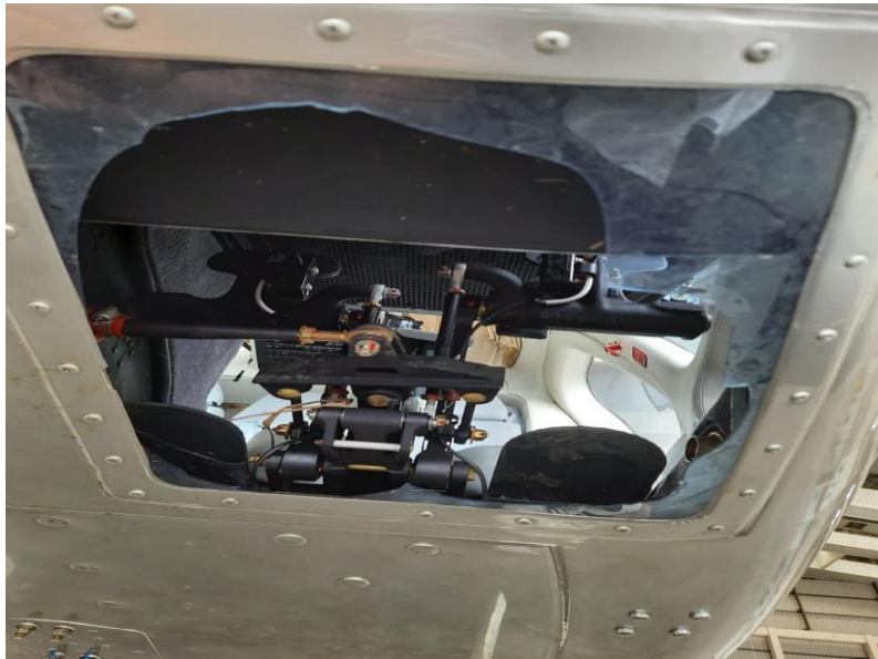
(Fig. 17: Both the chin bubbles (cockpit lower glass) found broken)
