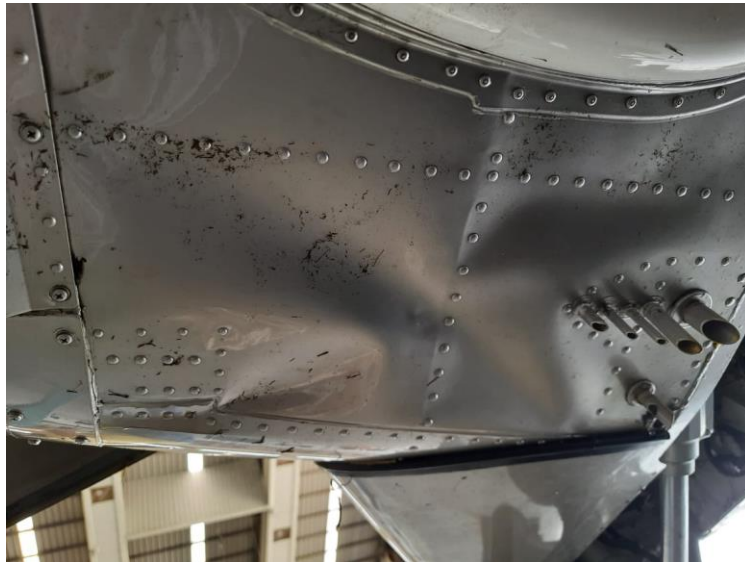
(Fig. 23: Belly, alongside vents line& Drain lines found Deformed)
