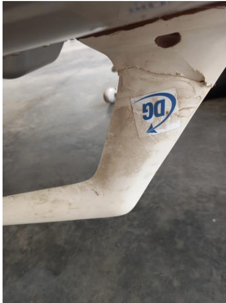
(Fig. 19: VHF 2 Antenna broken)
