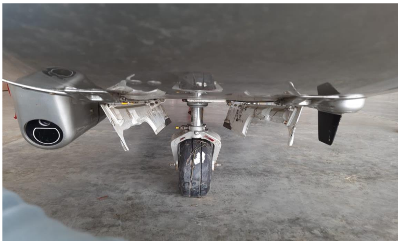
(Fig. 15: Nose Landing Gear doors twisted and broken)
