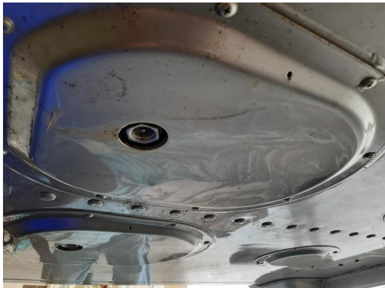
(Fig. 20: Utility accumulator access panel Deformed)
