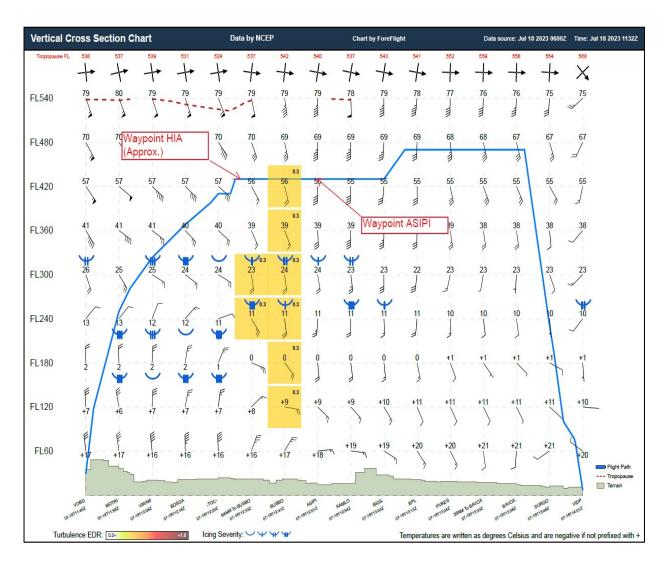
At top of climb short of waypoint HIA winds were about 30 knots from east south with temperature -57 degree Celsius at FL 420 at time 1220 UTC. Weather was there between short of waypoint BUSBO and waypoint ASIPI with light to moderate turbulence (turbulence EDR 0.3) at FL 430.
