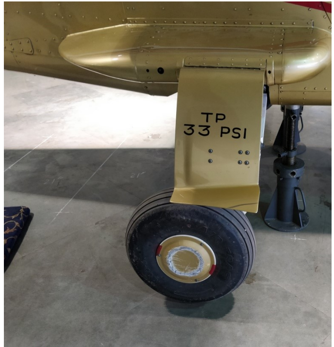
Scuffing damage on RH MLG Wheel
