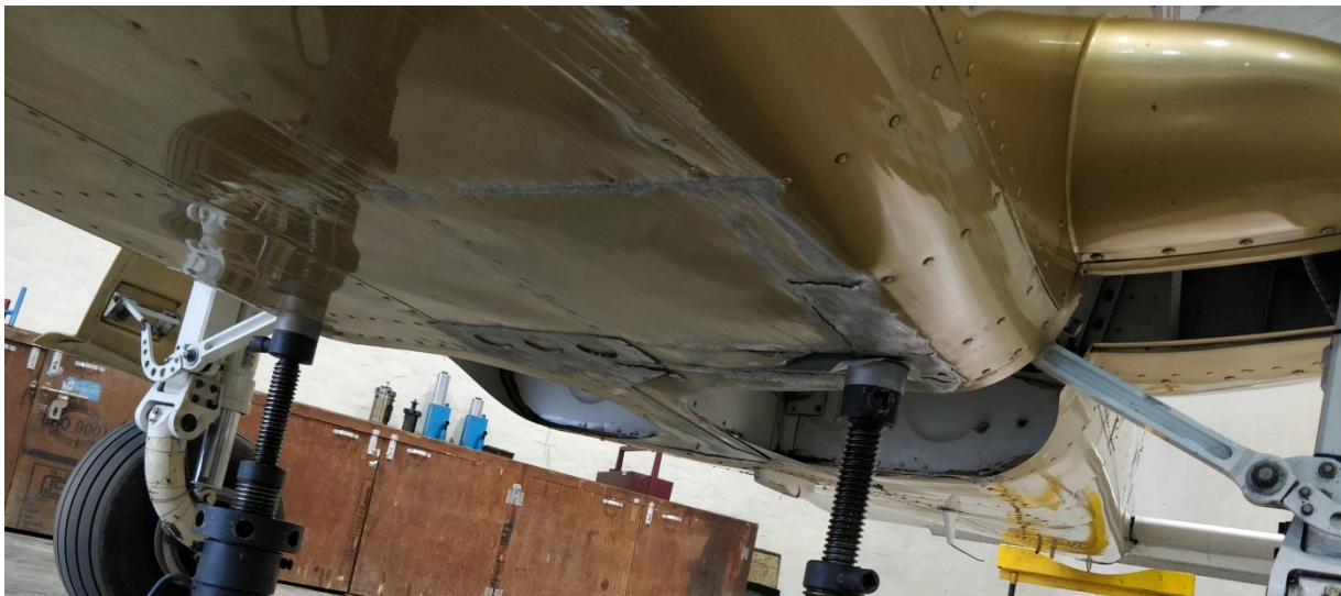
Damage to aircraft skin on the frame on LH side (13" FWD of aircraft datum) – Photograph taken from FWD looking AFT
