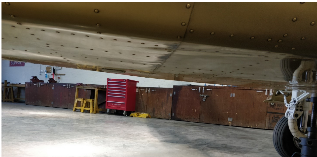
Damage to aircraft skin on the frame on LH side (23" FWD of aircraft datum) – Photograph taken from aircraft LH looking towards RH side
