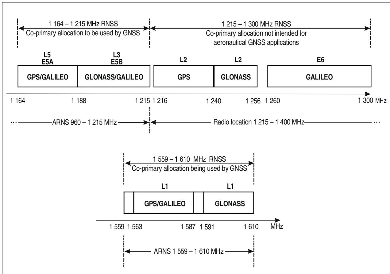
**Figure 6-1. GNSS spectrum**
