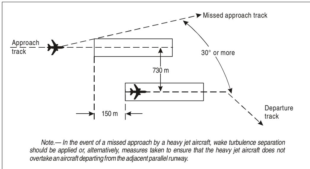
**Figure 4-2. Segregated parallel operations where runways are staggered**
