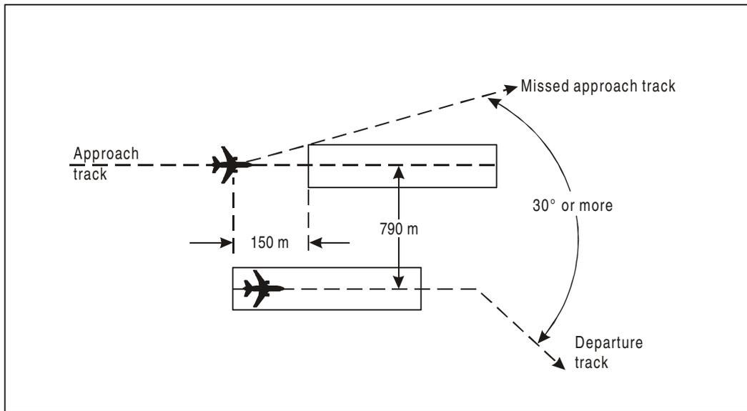
**Figure 4-3. Segregated parallel operations where runways are staggered**
