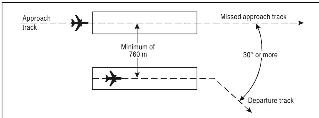
**Figure 4-1. Segregated parallel operations where thresholds are even**
