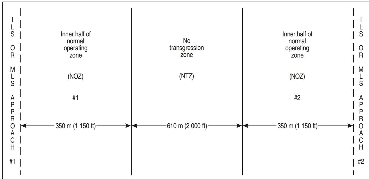
**Figure 2-2. Example of spacing of NOZs and NTZ**
