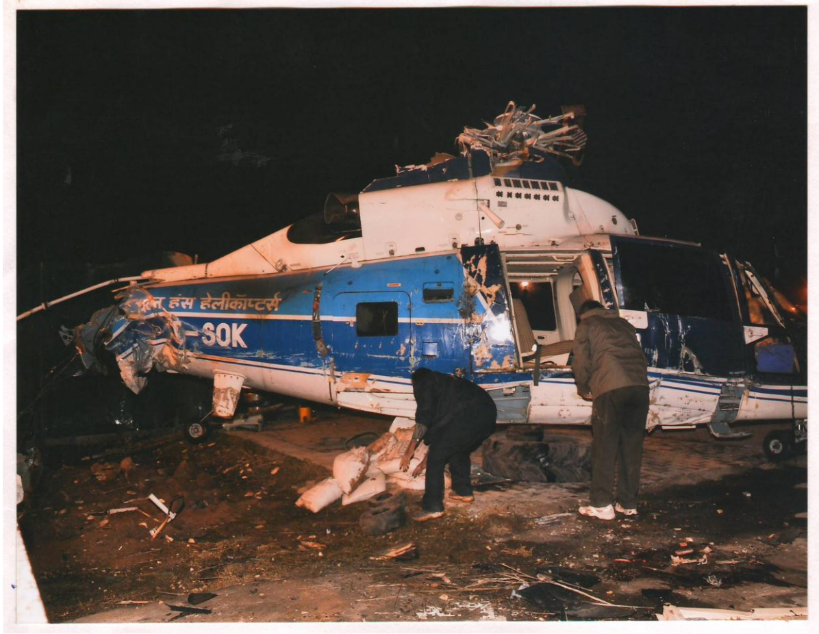
Picture: Side view showing damage on Right Side
